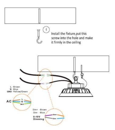
5 Hang on the light and connect the wire. Then light up to test
